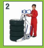
To grasp the tyres, press the handles outwards to close the scissor manipulator
