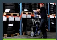
No more restacking. With the tyre truck, stacks of tyres can be taken directly from pallets.
